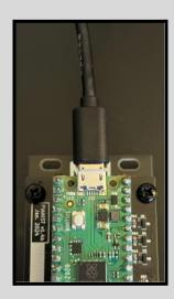
Install the <u>Thonny IDE</u> and connect to the Pi Pico by selecting it from the bottom right menu.
