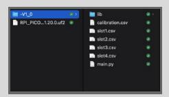
• If the Pi Pico is new you should see it as a peripheral device once plugged in. Go to the firmware folder and drag and drop the ".uf2" file onto the Pi Pico. This will install the correct version of MicroPython on the Pico (v1.20.0).
