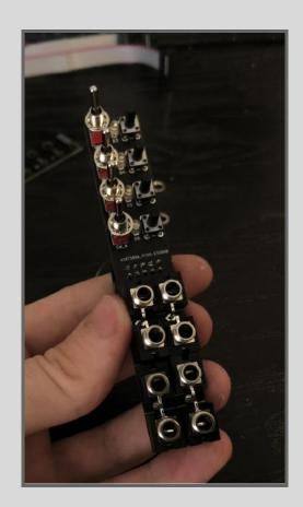
• Put the front panel and hand-tighten the nuts for each part. Be mindful that nothing has been soldered yet so components might disconnect or go out of place.
