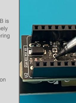
• Once all the components are properly soldered in place and double-checked, you can insert the male headers into both sockets, with the longer side of the header going in.
