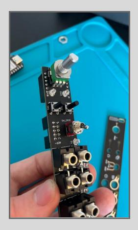
• Put the front panel on and hand tighten the nuts for the potentiometer, the switch, and all of the jack sockets
